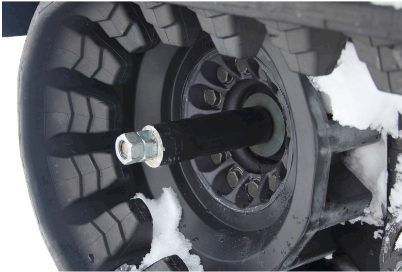
Figure 2: The improvised sprocket wheel repair.
