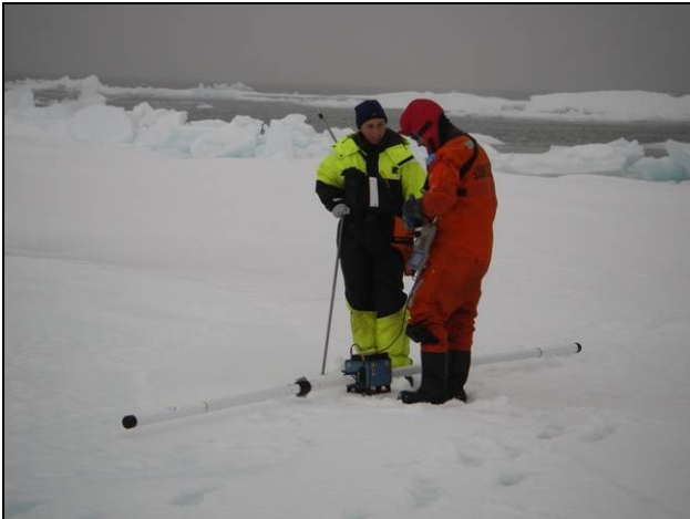
Figure 11: Use of the Geonics EM31 for indirect ice plus snow thickness measurements.
