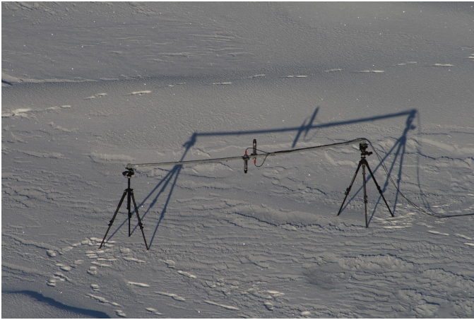
Figure 13: Albedo measurements, using two TriOS Ramses spectral radiometers, mounted on a 3m long pole between two tripods.
