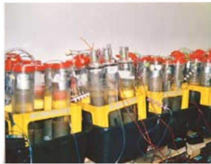
Measuring oxygen consumption in sediment communities
