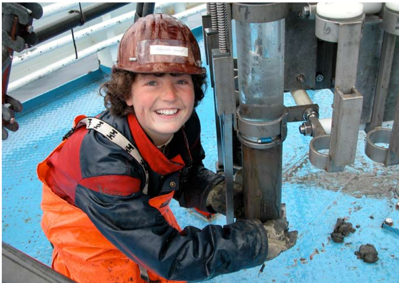
Student Silje Haaland from the University of Tromsø processes a multicore sample on deck. The multicore samples are used to investigate the sea bottom environment and the distribution of microfossils. Photo: Nalan Koç
