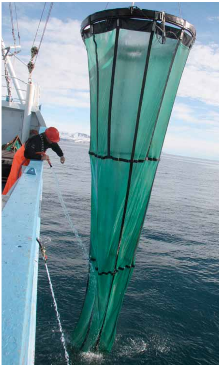
Sampling of zooplankton using a MIK net. Photo: Ole Magnus Rapp, Aftenposten
