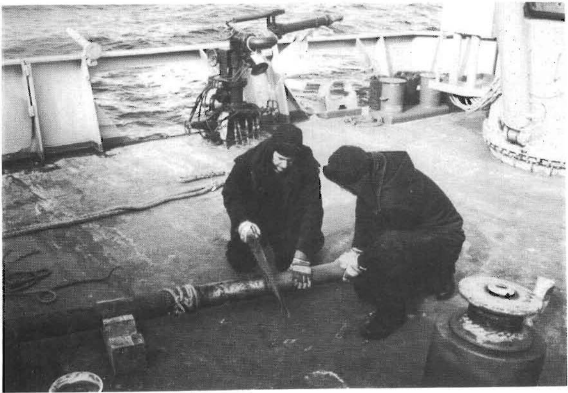
Fig. 2. Preparing the sampling device. A PVC tube is used as lining inside the steel tube for better sediment recovery.
