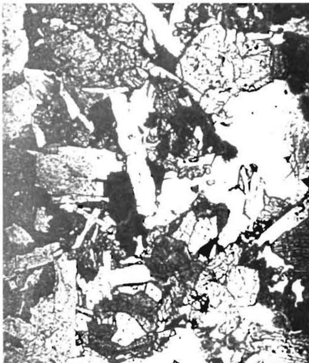
Fig. 5.2 Photomicrographs of basalts. 1 well-crystallised basalt with a rounded fragment of volcanic glass (typical of tholeiites) from the upper sheet on the Ciurlionis plateau, Hooker Island; thin section 278 (1957), x 16, plane light; 2 porphyritic-like hyalobasalt from the base of a thick sheet in the Cape Kavagli area, Salisbury Island, thin section 1089a (1957), x 28, plain light; 3 fine-grained olivine-bearing dolerite from a sill intruded between basaltic sheets which form Scott-Keltie Island, thin section 295a (1957), x 28, plain light.
