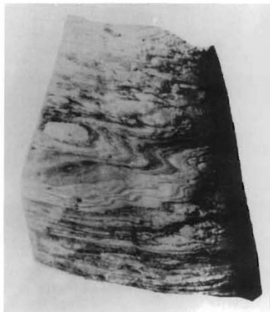
Fig. 3.1.4 Finely corrugated and lenticular, fine-grained quartz-sericite schist, with completely transposed, barrel-shaped boudins. Borehole depth 3143.7 m. Polished section, full size.
