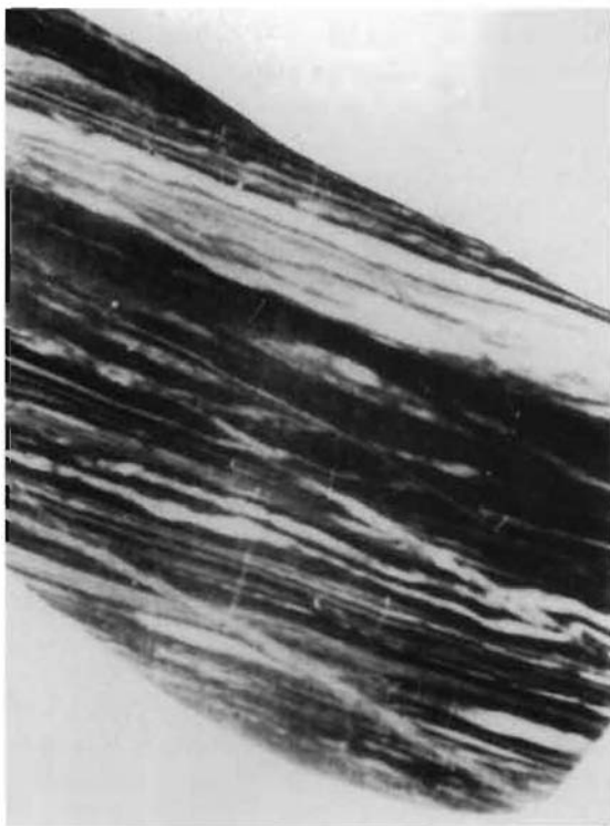
Fig. 3.1.2 Intercalated quartzite and fine-grained quartz-sericite schist. Borehole depth 3200 m. Full size.
