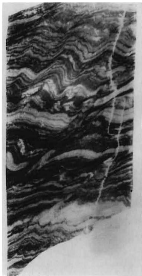
Fig. 3.1.7 Cleaved and folded, fine-grained quartz-sericite schist. Fissures filled with secondary calcite. Borehole depth 3046.3 m. Polished section, full size.
