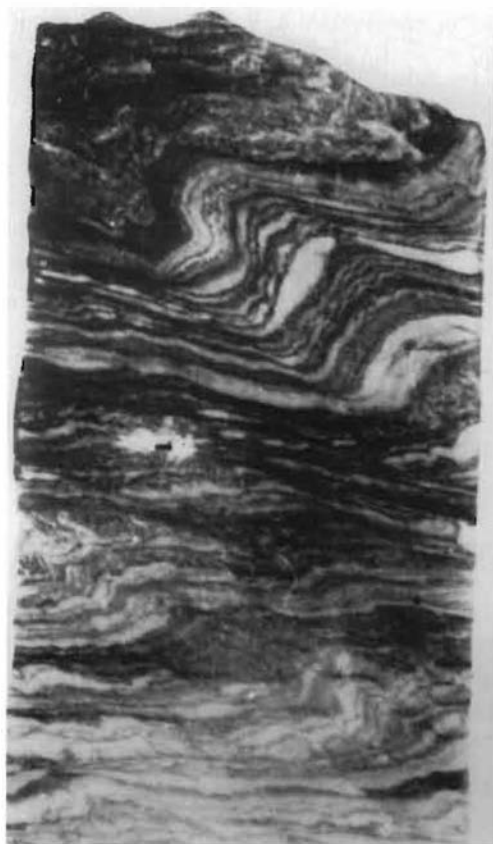
Fig. 3.1.3 Corrugated, fine-grained quartz-sericite schist (alternating, mainly micaeous and mainly quartzose material). Lenticular boudins consist of competent, fine-grained quartzite in an incompetent matrix of sericite schist. Borehole depth 3116.5 m. Polished section, full size.
