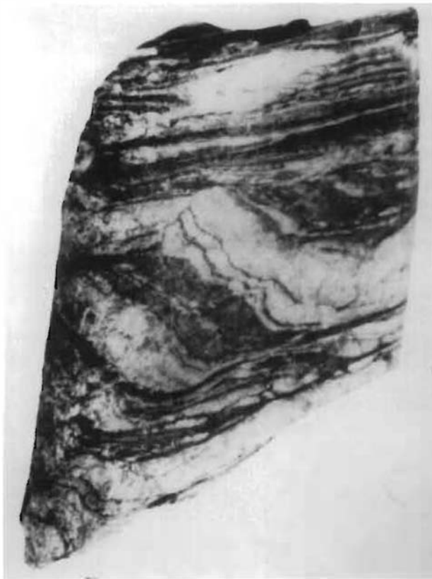
Fig. 3.1.8 Tectonic breccia composed of fragments of fine-grained quartzite in quartz-sericite schist. Borehole depth 3068.1 m. Polished section, full size.
