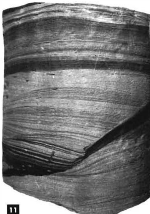
Fig. 4.2 Sedimentary structures: horizontal, lenticular-sinuuous and cross lamination with elements of flaser bedding, typical of alternating rocks in the upper parts of rhythms. 8 and 9 are upper Anisian from the Hayes borehole, depths 3194 and 3193 m; 10, 11 and 13 are upper Carnian from the Severnaya borehole, depths 1023 and 1022 m; 12 is upper Carnian from the Hayes borehole, depth 745.9 m. Polished core, full size.
