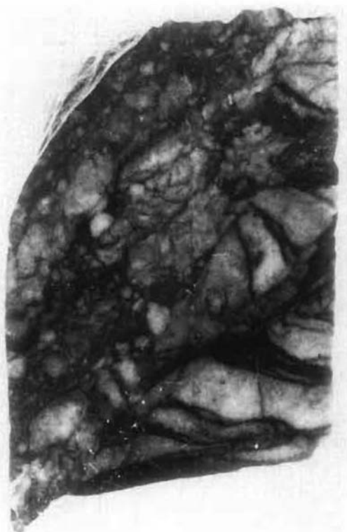
Fig. 3.1.6 Fine-grained schistose quartzite with small boudins. Borehole depth 2145 m. Polished surface, full size.
