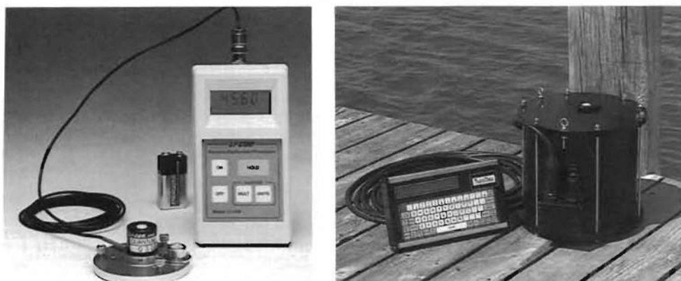
Figure 1: Photos of the LI-190SA and LI-189 (left), and the LI-1800UW (right).
