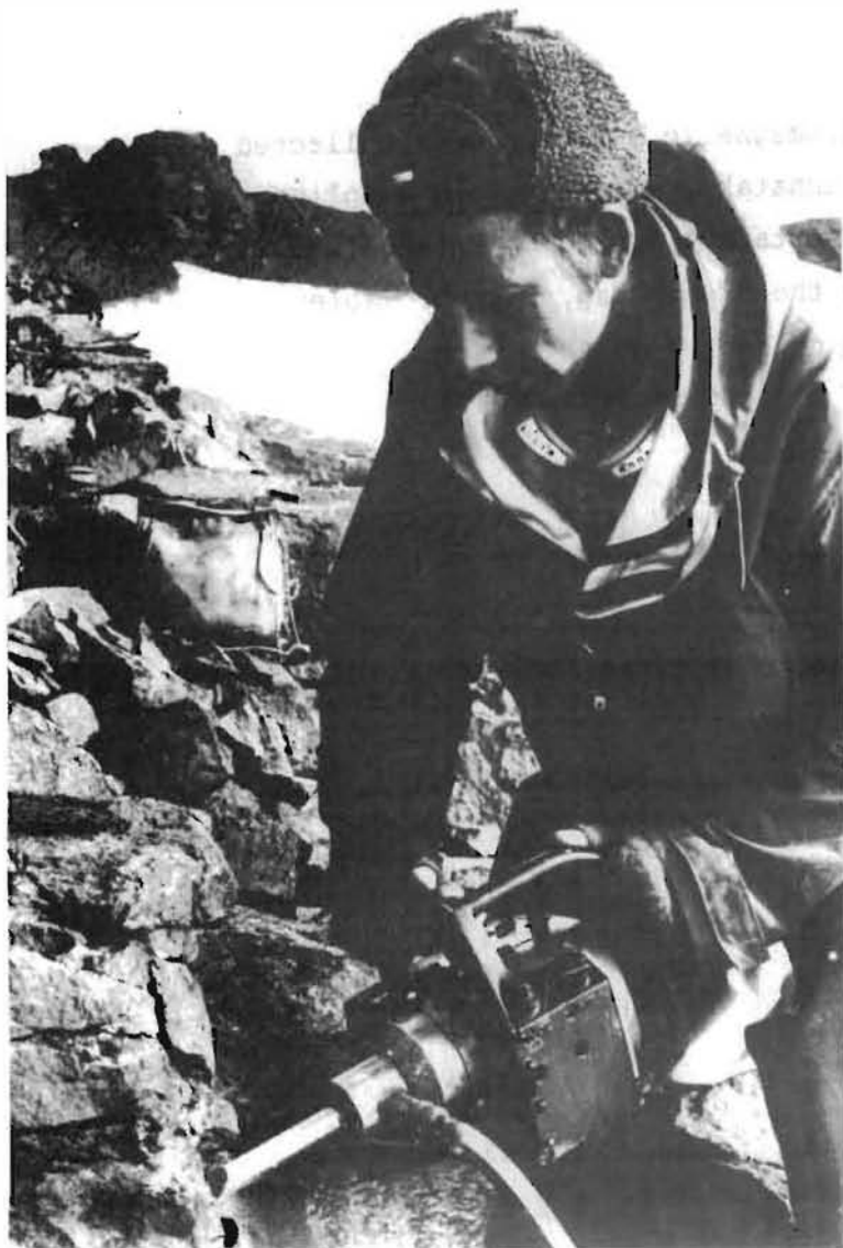
Fig.1. Field operation of motorized, water-cooled diamond corer.
