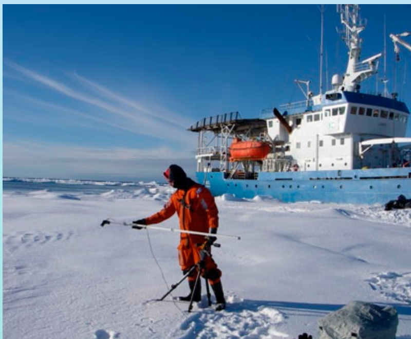
Optical measurement of albedo in the Fram Strait. Image: ©Sebastian Gerland, Norwegian Polar Institute
