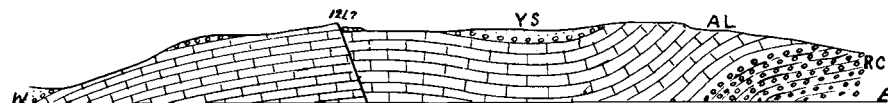
Fig. 35. Section showing the fault (same as in fig. 34) on the south side of Gluggdalen. RC Red Conglomerate, AL Ambigua Limestone, YS Yellow Sandstone.
