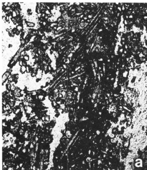
Fig. 22. a. Thin section of a chert pebble from the Brentskardhaugen Bed showing sponge spicules. Crossed nicols (x 51).
