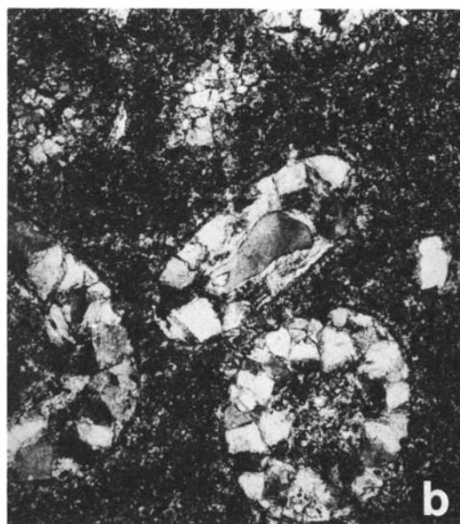
Fig. 22. a. Thin section of a chert pebble from the Brentskardhaugen Bed showing sponge spicules. Crossed nicols (x 51).
