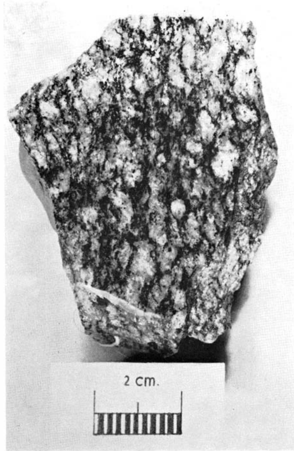
A. Lineated gneissose feldspahite of the Femmilsjøen member of the Bangenhuk formation.
