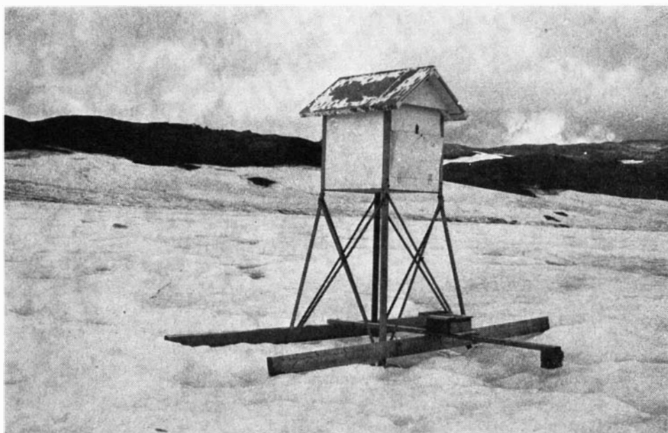
Fig. 18. Standard hut, containing one thermohygrograph and the usual meteorological thermometers, fixed at 170 cm above the glacier surface during the whole summer by the aid of a pillar arrangement of steel rods and planks.
