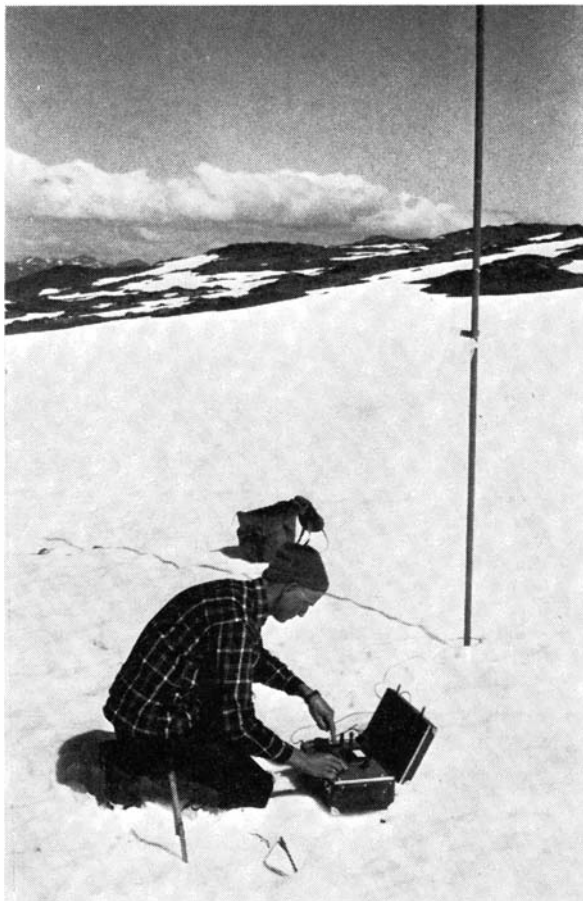
Fig. 13. The resistance (measured in ohms) for calibrated thermistors drilled down in the ice masses is registered with a model of Wheatstone's bridge.
