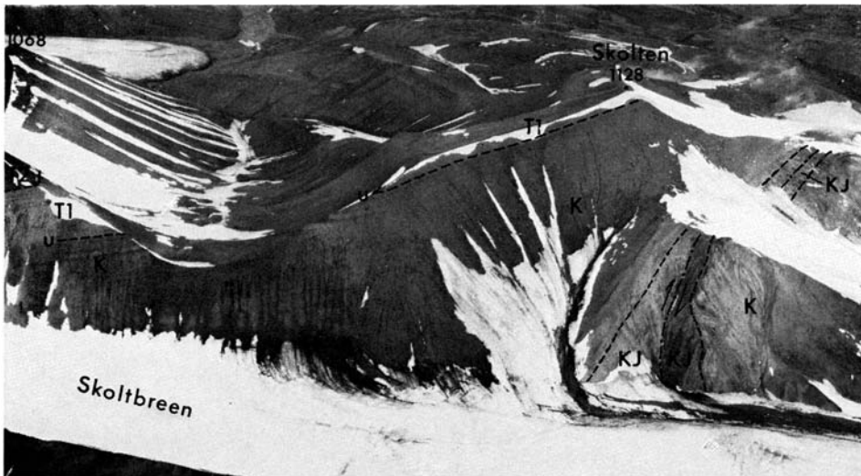
Fig. 11. Oblique aerial view (towards north-west) of Skolten showing the western line of the Billefjorden fault zone. The structure developed here is a faulted anticline with the Janusfjellet Formation (KJ) exposed in its crest. Other rock units exposed are: Helvetiafjellet and Carolinefjellet Formations (K), Firkanten Formation (T1) with unconformity (u) at base, Basilika and Sarkofagen Formations (T2).
