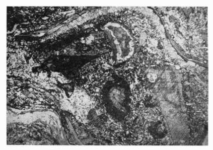
Fig. 33. Biocalcarenite. Fossil remains are in part silicified. Matrix consists mainly of minute siliceous sponge spicules. Brachiopod Cherts, Akseløya, thin-section A-10b, plane polarized light,  $\times 12.5$ .
