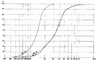
Fig. 11. Granulometric composition of the carbonate-cemented quartz sandstones from the Tokrossøya Beds on Sørkappøya.
