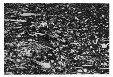
Fig. 29. Calcareous spiculitic chert. Note planar arrangement of the sponge spicules. Brachiopod Cherts, Bellsund, W of Sundodden, thin-section S-45-65, plane polarized light, ×50.
