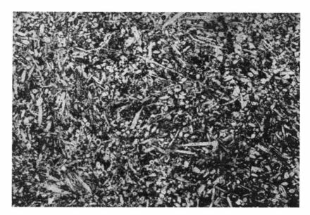
Fig. 25. Spiculite. Sponge spicules consist of chalcedony; matrix is stained by pyrite, iron-oxides and carbonaceous matter. Brachiopod Cherty Limestone, Hornsund, Treskelen, thin-section P-3, plane polarized light, ×31.2.
