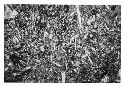
Fig. 34. Biocalcarenite. Bryozoan fragments prevail. Minute siliceous sponge spicules are the predominant component of the matrix. Brachiopod Cherts, Akseløya, thin-section A-10d, plane polarized light, ×12.5.
