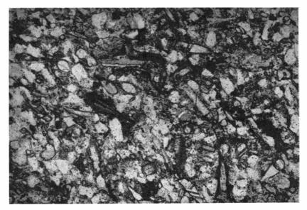
Fig. 23. Arenaceous calcareous spiculitic chert. Sponge spicules either consist of chalcedony or are calcified. Lower Tokrossøya Beds, Øyrlandet, Øyrlandsodden, thin-section Ø-15, plane polarized light, × 50.
