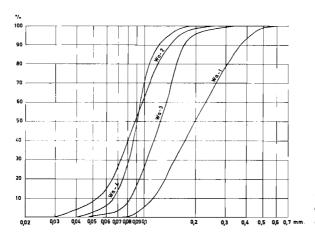
Fig. 14. Granulometric composition of the fossiliferous, calcareous sandstones and siltstones from the Tokrossøya Beds on Sørkappøya.
