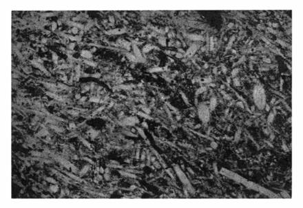
Fig. 10. Arenaceous calcareous spiculitic chert. Sponge spicules consist mostly of chalcedony; their outlines are poorly defined. Matrix consists mainly of carbonates and fine-crystalline brownish silica. Lower Tokrossøya Beds, Tokrossøya, thin-section Pk-22b, plane polarized light, × 50.
