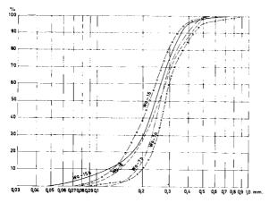
Fig. 12. Granulometric composition of the quartzitic sandstones from the Tokrossøya Beds on Sørkappøya,
