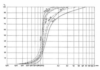
Fig. 7. Granulometric composition of the fossiliferous, calcareous sandstones and siltstones from the Tokrossøya Beds on Tokrossøya.
