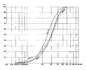
Fig. 4. Granulometric composition of the carbonate-cemented quartz sandstones from the Tokrossøya Beds on Tokrossøya.
