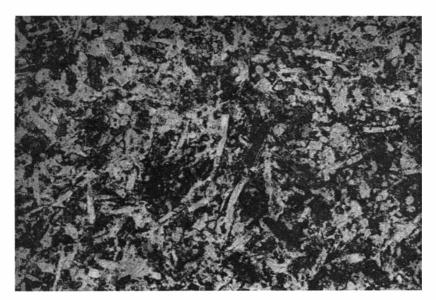
Fig. 28. Calcareous, fossiliferous spiculitic chert. Sponge spicules consist of chalcedony. Matrix consists of fine-crystalline silica and scattered carbonate rhombs. Brachiopod Cherts, Akseløya, thin-section A-8b, plane polarized light, × 50.
