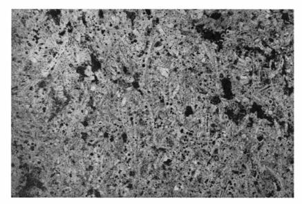
Fig. 32. Spiculite, Sponge spicules with poorly defined outlines consist of chalcedony. Fine-crystalline siliceous matrix comprises scattered carbonate rhombs and pyrite. Brachiopod Cherts, Akseløya, thinsection A-8a, plane polarized light,  $\times 50$ .
