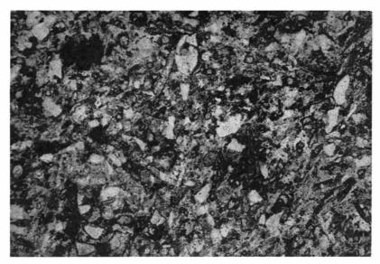
Fig. 18. Arenaceous calcareous spiculitic chert. Outlines of the chalcedony spicules are poorly defined while the calcified spicules are distinct. Lower Tokrossøya Beds, Sørkappøya, thin-section Wa-34, plane polarized light, ×50.
