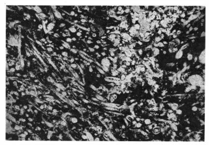
Fig. 27. Calcareous fossiliferous spiculitic chert. Sponge spicules consist mostly of chalcedony; matrix consists of fine-crystalline silica and carbonates. Brachiopod Cherts, Akseløya, thin-section S-40-65, plane polarized light, × 50.
