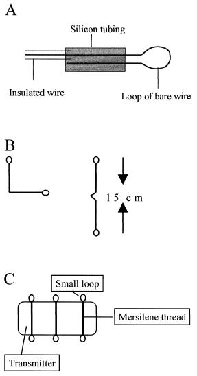
Figure 1. Illustration of how the electrode wire's distal end was prepared to form a nonopening loop before implantation A. Illustration of the two different electrode placements under the skin. B. Illustration of how the three parallel mersilene thread belts were formed around each transmitter, showing the position of the small mersilene loops on opposite sides of the transmitter, which were used as anchoring points to facilitate attachment to the abdominal wall C.
