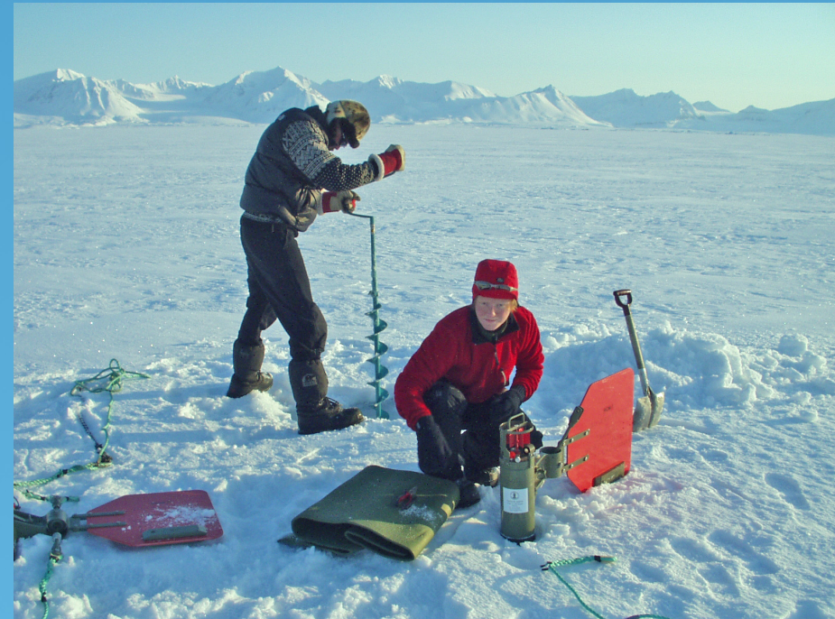
Deployment of current meters below the fast ice at Kongsfjorden, Svalbard. Water current below the sea ice are crucial for energy fluxes at the ice-ocean interface, and within that for freezing and melting processes. Photo: Sebastian Gerland
