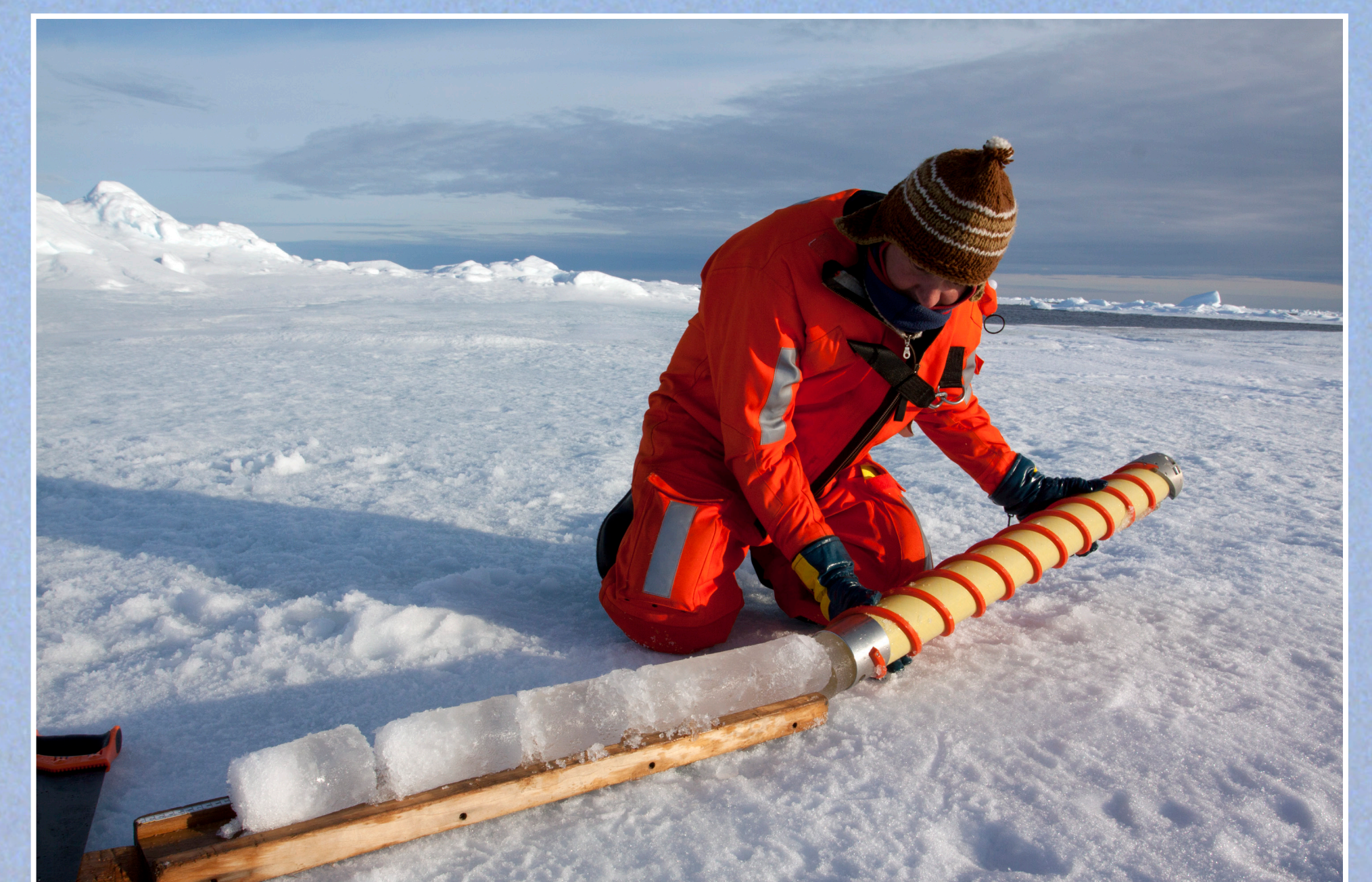
Sea-ice scientist Sebastian Gerland is removing a sample of sea ice taken with a corer drill. Several metres of core can be obtained from the sea ice, revealing its physical properties and details about its chemistry and biology, including algae that grow in the ice. Photo: Tor Ivan Karlsen
