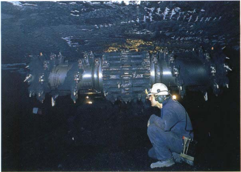
Fig. 26 Electrical cutter eating its way into the coal seam. Gruve 7 (Mine 7), Longyearbyen.
