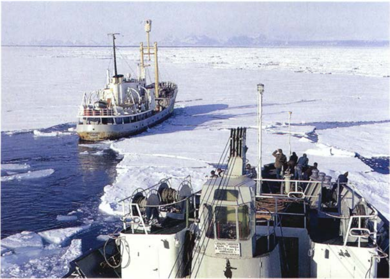
Fig. 51. Following a persistently cold winter, the fjord ice may be so solid that it poses a hindrance to shipping well into the summer. Here, a sealer, specially strengthened to penetrate ice, is breaking a lane for a passenger ship on its way to Longyearbyen. (V.H.)
