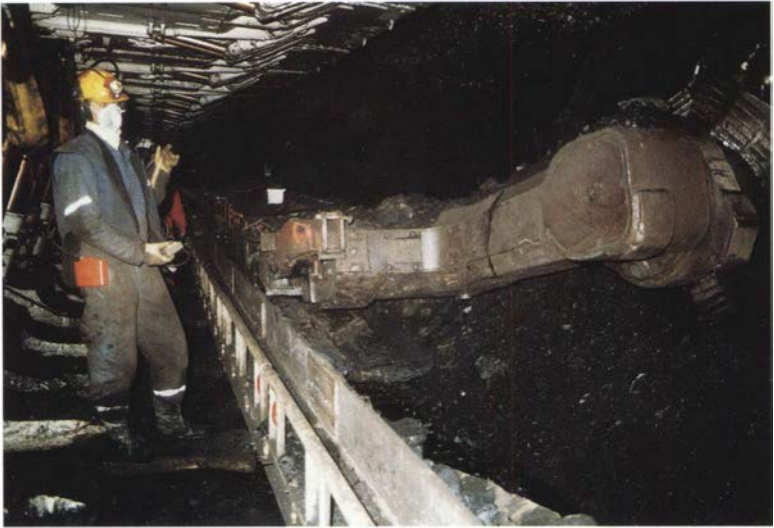
Fig. 102. Modern mining machinery excavating coal in Sveagruva. The seams here are significantly thicker and working conditions therefore much simpler than in the mines at Longyearbyen. There the seams to a large extent are less than 1 m thick and work often has to take place lying down or kneeling. (S.H.)
