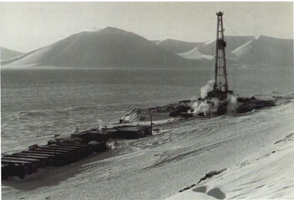
Fig. 89. In the mid-1960s, American Overseas Petroleum Ltd. drilled for oil at Blåhuken on the north coast of Van Mijenfjorden. A depth of 3.3 km was reached, but no oil was encountered, just traces of gas of no commercial interest. Several other attempts have been made to find oil in Svalbard, all in vain. (H.G.)
