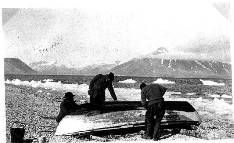
Caulking the dory, "Bruce City". L. to r.: Longstaff, Walton, C.S.E. Patunia Bay beyond.
