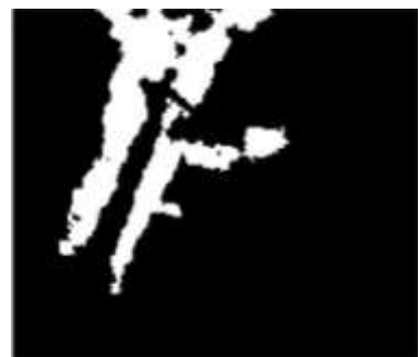
Figure 3: Automatic detection applied on RADARSAT-2 UF mode images from 2013.06.10 and 2013.09.14. A threshold of 2.5db, followed by a filter to eliminate speckle is applied on the difference in backscatter of the two images.
