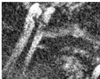
Figure 2: RADARSAT-2 UF mode image from 2013.06.10 at Dryadreen, Svalbard. Showing a bright tongue-shaped feature consistent with an avalanche debris field.
