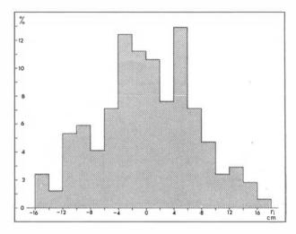
FIG. 2. — Frequency distribution of the difference between observed and computed heights of the tide  $(r_4)$ .
