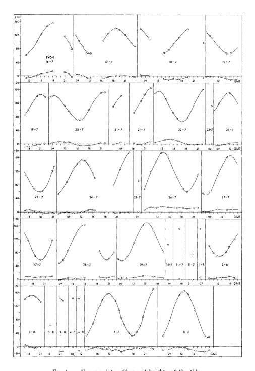
FIG. 1. — Upper points : Observed heights of the tide. Lower points (close to the zero line) : Difference between observed and computed tides  $(r_4)$ . Points separated by time intervals less than three hours are connected by smooth curves.
