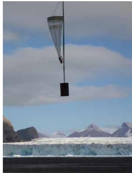
Top: Helicopter ready for takeoff with the bottle-rosette to take water samples. Bottom: Instruments were attached to a weighted 110-metre line suspended below the helicopter. Photos: Harald Steen / Norwegian Polar Institute
