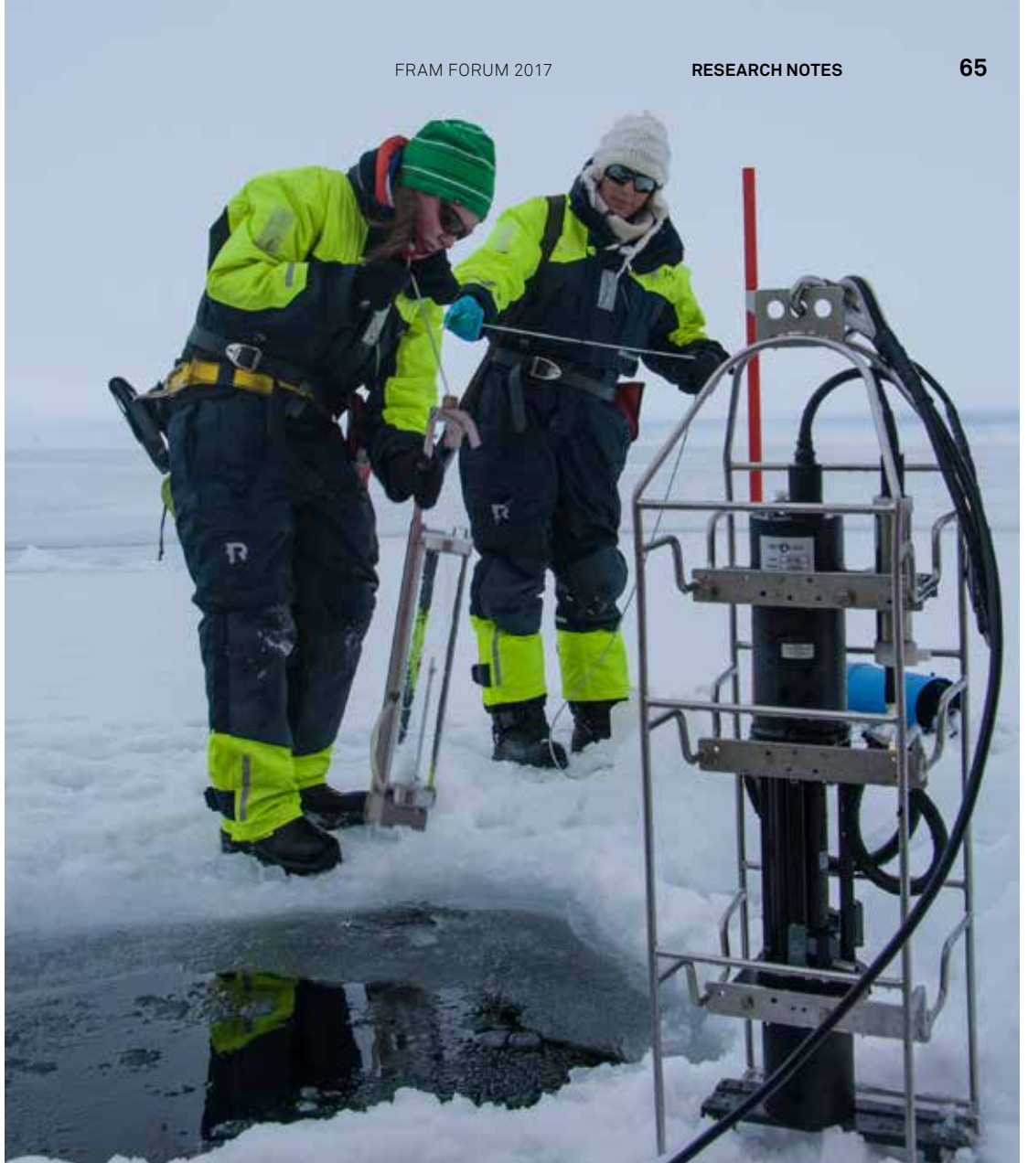
Sampling the optical properties of the water column through a hole in the thin ice of the refrozen lead.
