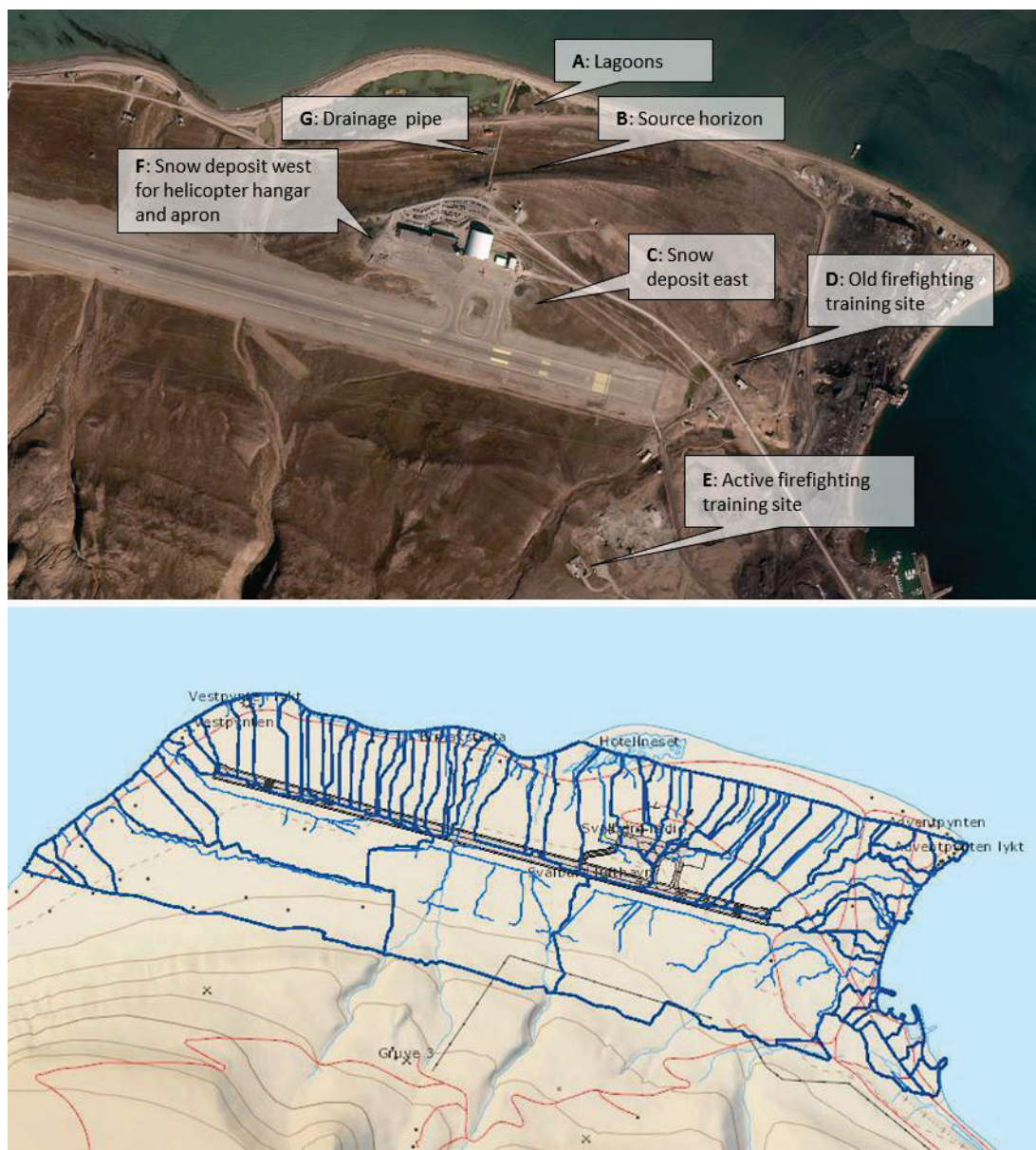
Figure 3. Radar image of the Longyearbyen air- and heliport (top) with some installations and sites associated with handling or storage of hazardous materials indicated: A) lagoons, B) source horizon, C) snow deposit east, D) old firefighting training site, E) active firefighting training site, F) snow deposit west for helicopter hangar and apron, and G) drainage pipe. Radar image courtesy the Norwegian Polar Institute. Bottom map showing land runoff water drainage around the Longyearbyen Airport (Pengerud & Kvisle, 2016).
