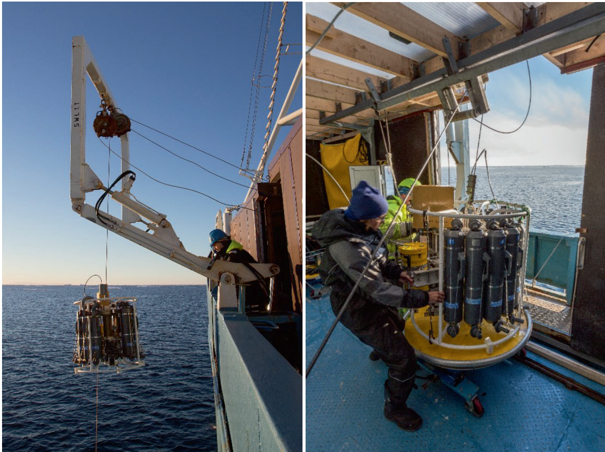
Collecting CTD measurements from the West Spitsbergen Current during the Norwegian Polar Institute's 2016 Fram Strait cruise. The Fram Strait CTD section has been repeated annually since 1997 as part of the Fram Strait Arctic Outflow Observatory. Photos: Paul A. Dodd, Norwegian Polar Institute.
