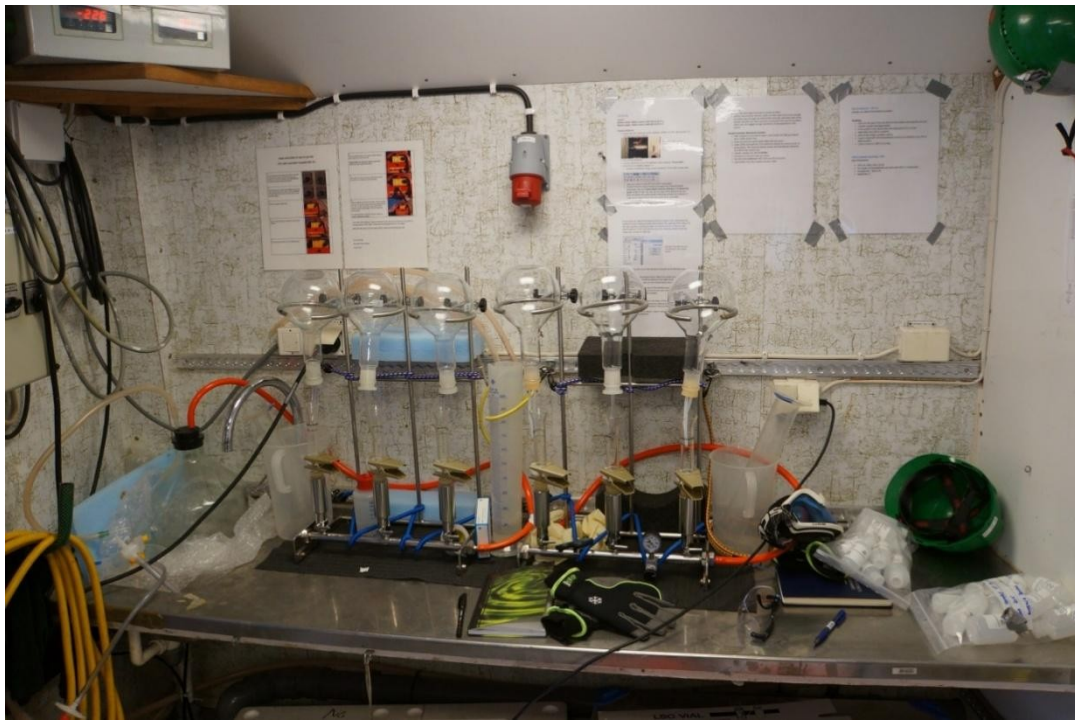
Figure 14: Filtration equipment for water samples in the laboratory onboard.
