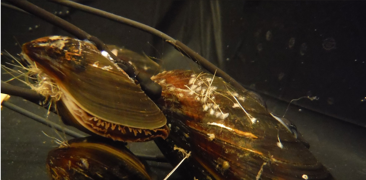
Icelandic scallops (top) and blue mussels (bottom) are ready to be deployed in the field with the electrodes glued onto their shells. Photos: Damien Tran
