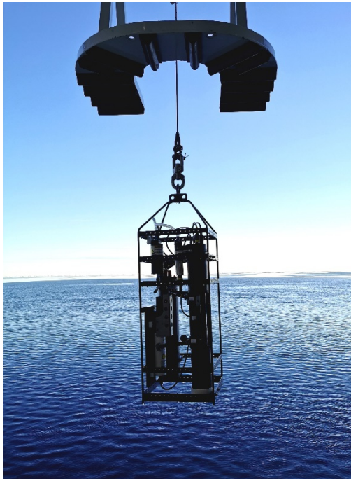
Figure 8.1 - Deployment of the optics cast from the CTD hangar of RV Kronprins Haakon
