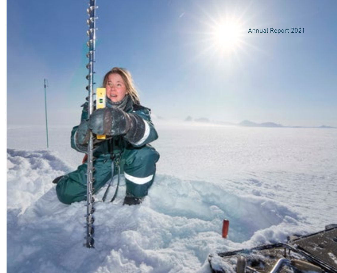
ICE MASS BALANCE Glaciologist Emily Geyman carrying out fieldwork on the Holtedahlfonna glacier in Svalbard, aimed at measuring the mass balance. The mass balance of a glacier is the difference between growth due to precipitation in winter and reduction in summer as a result of melting and runoff. Photo: Stein Tronstad / Norwegian Polar Institute
