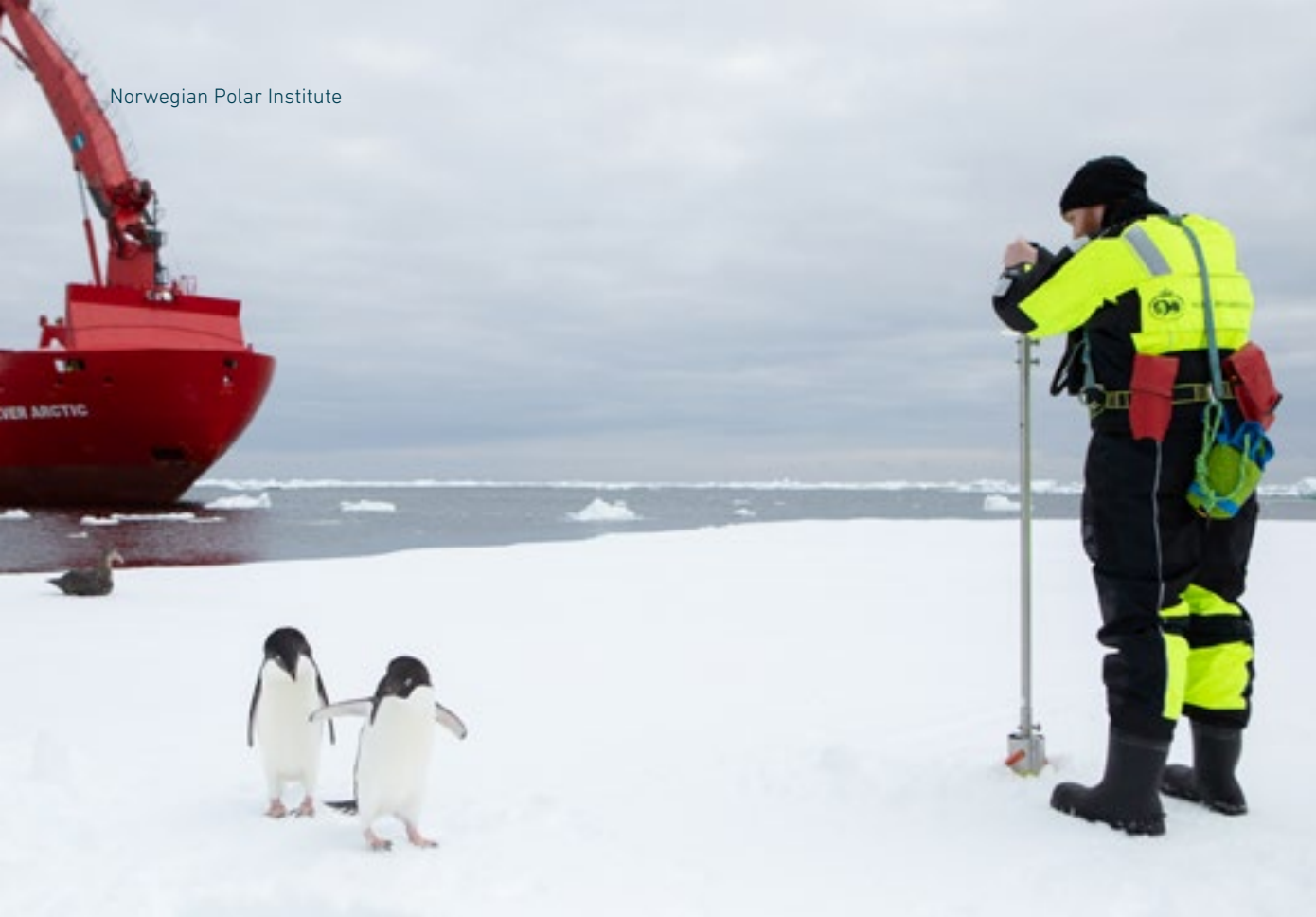
RESEARCH An ice core is extracted from the sea ice in the Southern Ocean, Dronning Maud Land. These ice cores provide information about biochemical processes in the ocean. A southern giant petrel and Adélie penguins look on. Photo: Samuel Martínez Llobet / Norwegian Polar Institute
