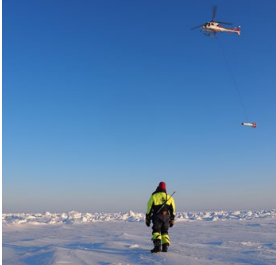
SEA ICE STUDIES A helicopter measures the thickness of sea ice on the Arctic Ocean using an electromagnetic instrument during the winter expedition of 2021 as part of The Nansen Legacy project. A number of researchers and technicians from the Norwegian Polar Institute took part. Photo: Adam Steer / Norwegian Polar Institute
