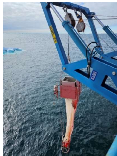
Figure 6.1: Multinet deployed from A-frame during TT24.
