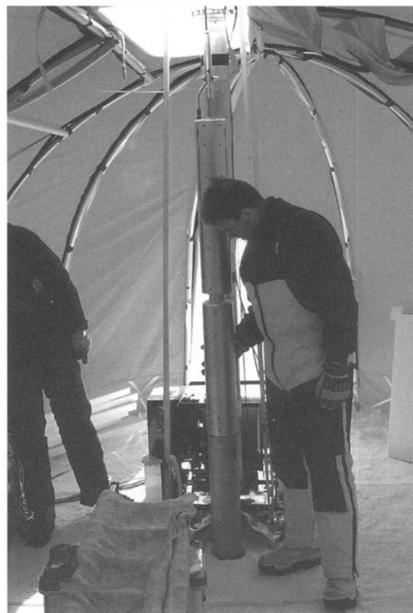
Fig. 2 The drill used for the medium long cores
