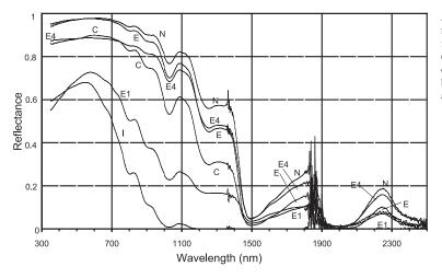
*Fig. 2.* Reflectance curves of new snow (N), equilibrium forms (E), equilibrium forms (40 mm) on basal ice (E4), equilibrium forms (10 mm) on basal ice (E1), bare basal ice (I) and melt–freeze crust (C).
