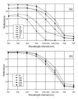
*Fig. 4.* Reflectance values re-sampled in discrete wavelength intervals: (a) equilibrium forms (E, E4, E1), basal ice (I), melt–freeze crust (C); (b) drifted snows (SD, DB, DR and DE). New snow (N) is shown in both plots.
