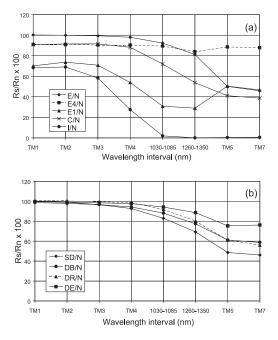
*Fig.* 5. Reflectance values (Rs) re-sampled in discrete wavelength intervals and normalized with respect to new snow reflectance (Rn): (a) equilibrium forms (E, E4, E1), basal ice (I), melt–freeze crust (C); (b) drifted snows (SD, DB, DR and DE).
