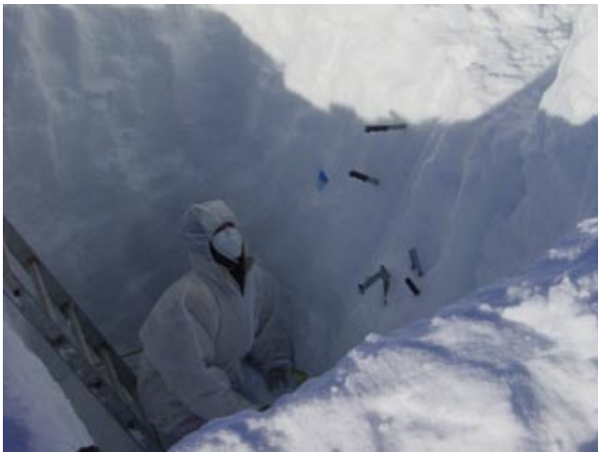
Fig. 3. Snow sampling for PCB studies on Lomonsovfonna, Svalbard. The white suit is important to prevent contamination of the samples with particles from field clothing.
