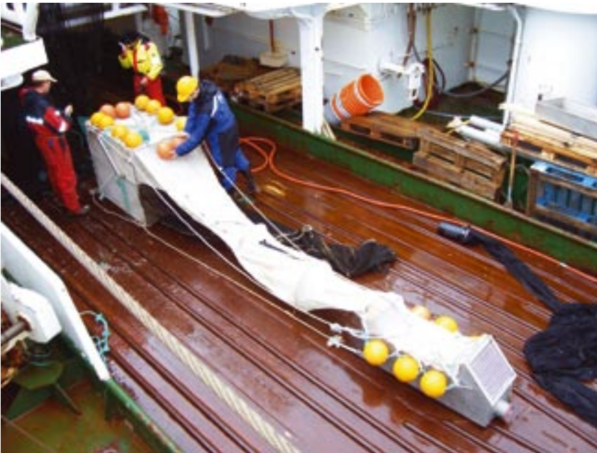
The live-fish-box employed for catching live polar cod in Kongsfjorden at 300 m depth. Photo: Lionel Camus.
