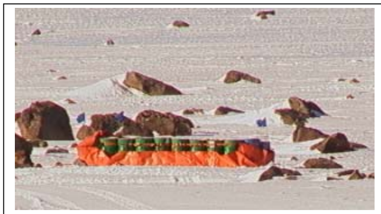
Figure 5: Fuel depot at Tor utilizing containment mats
