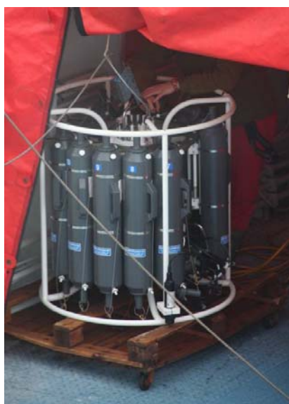
Figure 2. CTD-rosette used for water sampling. Photo: Guttorm N. Christensen, Akvaplan-niva.
