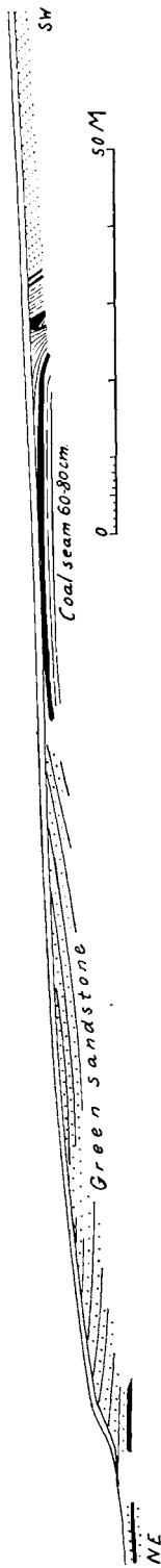
Fig. 42. Section along the eastern side of the creek in Brøggerdalen showing the Ragnhild Seam.
