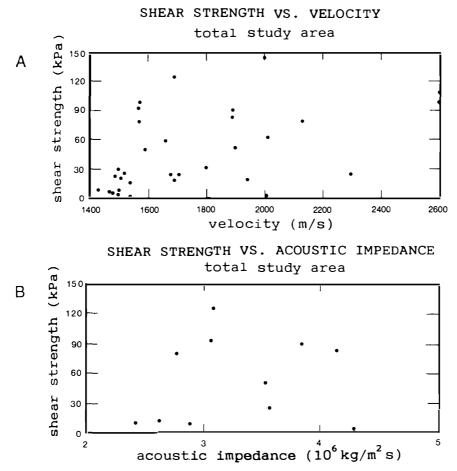
Fig. 28. Plots of undrained shear strength. A. Undrained shear strength versus compressional velocity. B. Undrained shear strength versus acoustic impedance.
