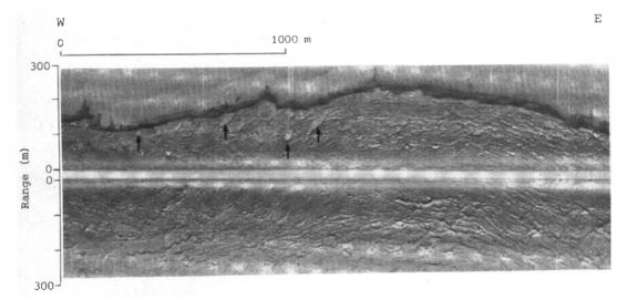
Fig. 12. Side-scan sonograph of the discontinuous, arcuate ridges subparalleling the ice front. Some possible iceberg calving impact features are marked with arrows. For location, see Fig. 10.
