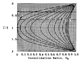
*Fig. 36.* Consolidation as a function of depth and time factor. From Taylor (1942). z = depth to sample. H = total drainage distance.
