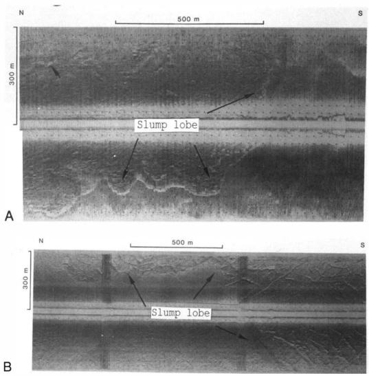
*Fig.* 8. A and B. Side-scan sonographs showing slump lobes on the distal part of the surge moraines. Note that the slumps cover pre-existing relief. Note also the small disturbances in the smooth slump lobe surface, and the possible detachment scars (short arrow) in A. For location, see Fig. 10.
