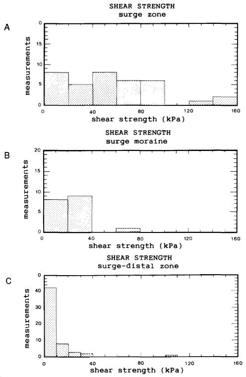
*Fig. 21.* Frequency histograms of undrained shear strength off Bråsvellbreen (pocket penetrometer and fall-cone) A. In the surge zone. B. On the surge moraine. C. Outside the surge moraine.
