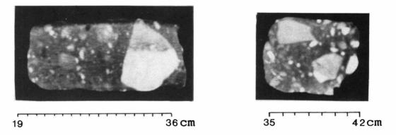
Fig. 19. Computer tomographs of two core samples from the surge zone. Note that the highest density has the lightest colour. For location, see Fig. 5C.
