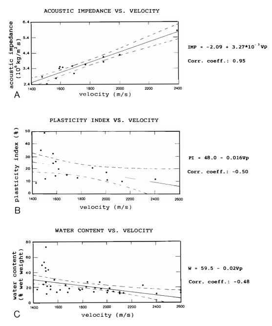
*Fig.* 27. Correlation between acoustical and other physical parameters. A. Acoustic impedance versus compressional velocity. B. Plasticity index versus velocity. C. Uncorrected water content versus velocity. D. Plasticity index versus acoustic impedance. E. Uncorrected water content versus acoustic impedance. F. Bulk density versus acoustic impedance. Correlation is done by simple, linear regression analyses. 95% confidence limit is shown by stippled lines.
