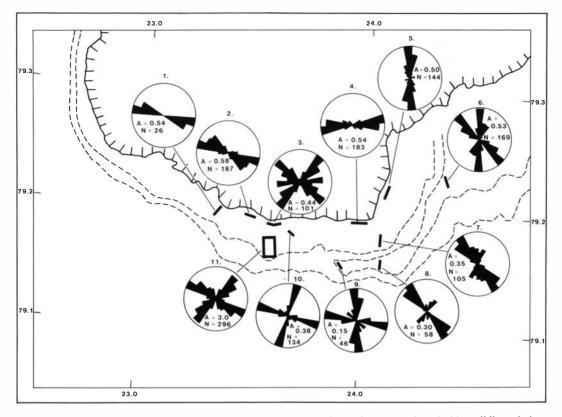
Fig. 11. Rose diagrams of directions of ridges in the surge zone. The analyses were done inside a sliding window of  $100 \times 200$  m across each area. N = number of counts. A = measured area in km<sup>2</sup>.
