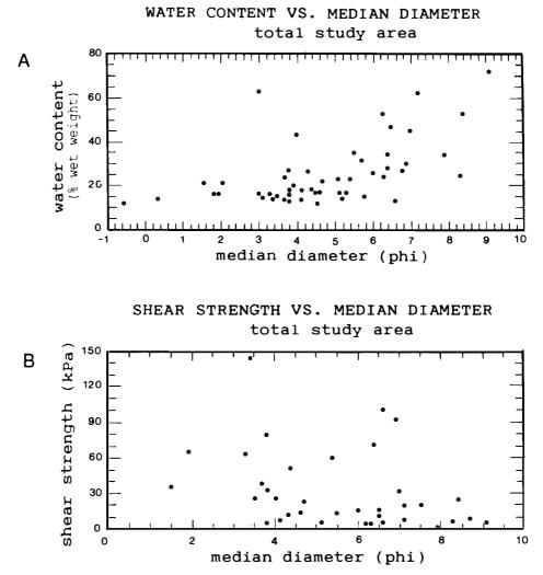
Fig. 26. Physical parameters plotted versus median grain diameter. A. Uncorrected water content. B. Undrained shear strength. C. Plasticity index. D. Acoustic impedance. E. Compressional velocity.
