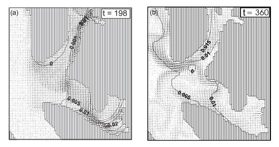
*Fig. 12.* Simulated surface circulation pattern: freshwater and up-fjord wind-driven with the same run-off and wind speed as in Fig. 10 after (a) 198 hours and (b) 360 hours of simulation time. The wind forcing is present in the period of 192-240 hours. The Surface height coutours are given in 0.005 m intervals.
