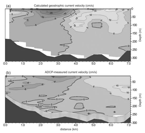
Fig. 14. (a) Calculated baroclinic geostrophic and (b) ADCP-measured current distribution at a section across the middle basin of Kongsfjorden, measured in July 1999. Positive values are up-fjord.
