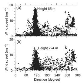
*Fig. 4.* Scatter plot of the wind speed versus the wind direction during ARTIST (Arctic Radiation and Turbulence Interaction Study) given by the sodar for (a) 65 m and (b) 214 m altitude. (from Argentini et al. 2000; printed with permission of the author and the Societa' Italiana di Fisica; copyright Societa' Italiana di Fisica))
