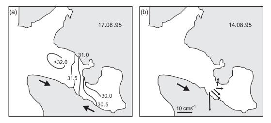
*Fig. 13.* (a) Surface salinity distribution and (b) surface current during a period with up-fjord wind in 1995. The heavy arrows on land represent the wind conditions during the mapping (rough scale:  $1 \text{ cm} = 4 \text{ m s}^{-1}$ ).
