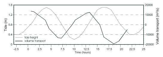
*Fig. 15.* Time series of tidal height and net volume transport across the constriction between the inner and outer parts of Kongsfjorden, measured in July 1999.
