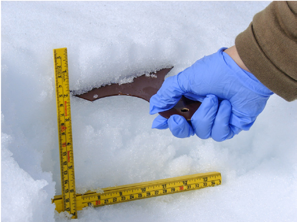
Fig. 4: Sampling surface snow using spatula and ruler (Picture C.A. Pedersen)
