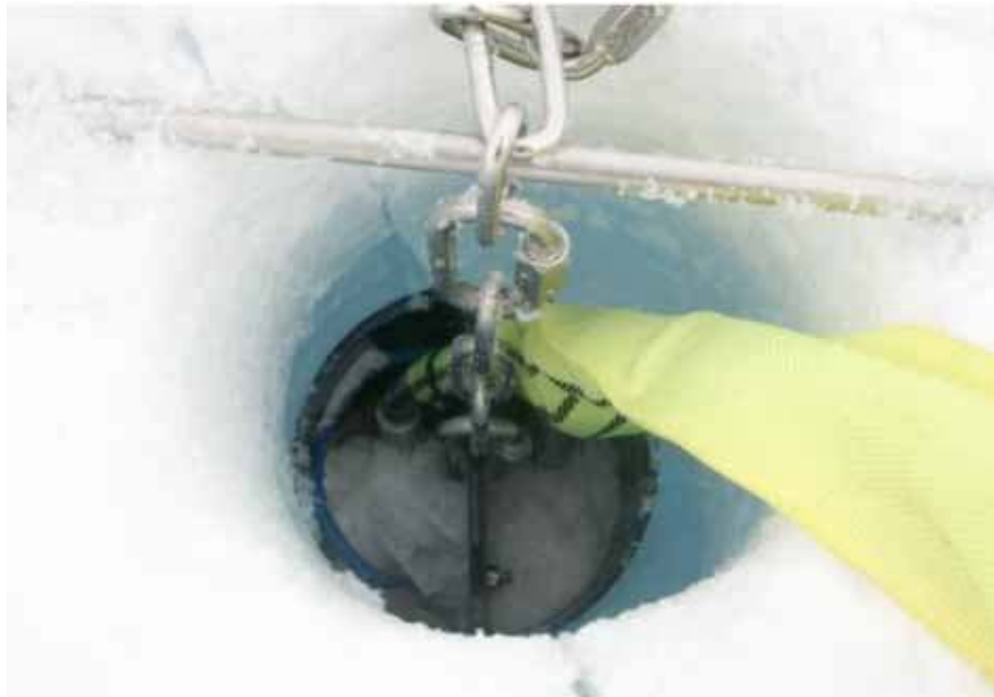
Figure 7.12: Borehole hydraulic jack lowered down into a borehole.
