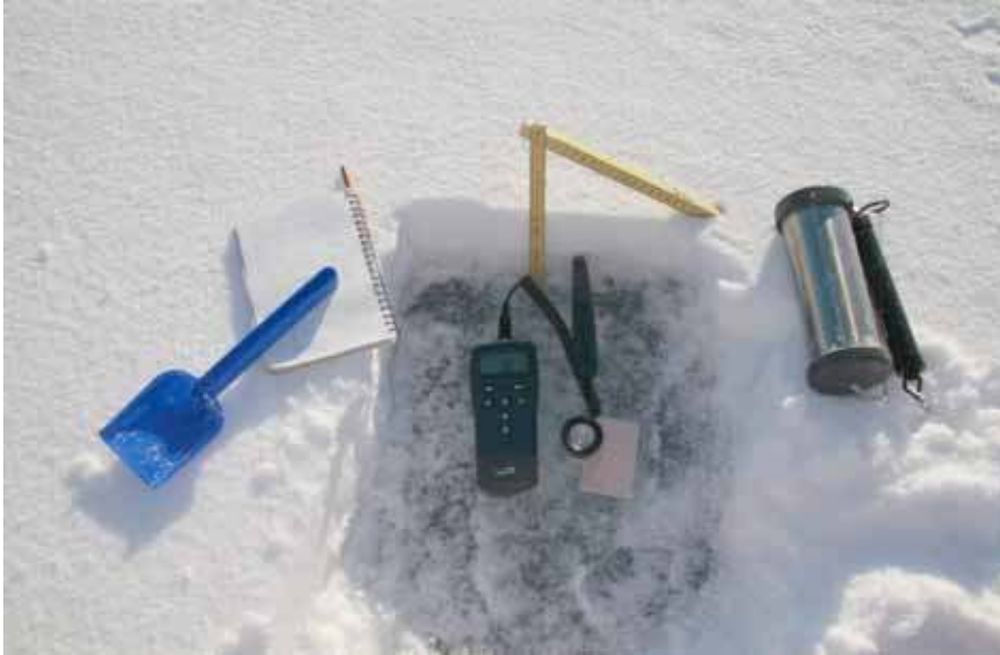
Figure 7.4: Example of snow pit stratigraphy and instruments.
