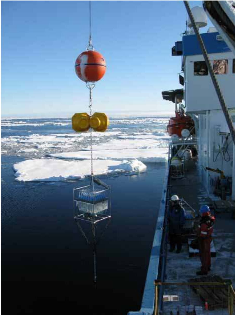
Figure 6.9: RAS 12239-02 being deployed anchor-first at mooring F17. A Microcat temperature and salinity instrument has been attached to the top of the frame containing the RAS.
