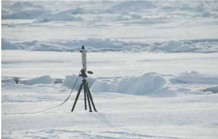
Figure 7.5: Using an upwards looking TriOS Ramses spectral radiometer for incoming radiation
