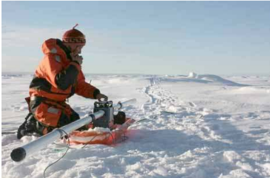
Figure 7.3: Use of the Geonics EM31 for indirect ice plus snow thickness measurements.
