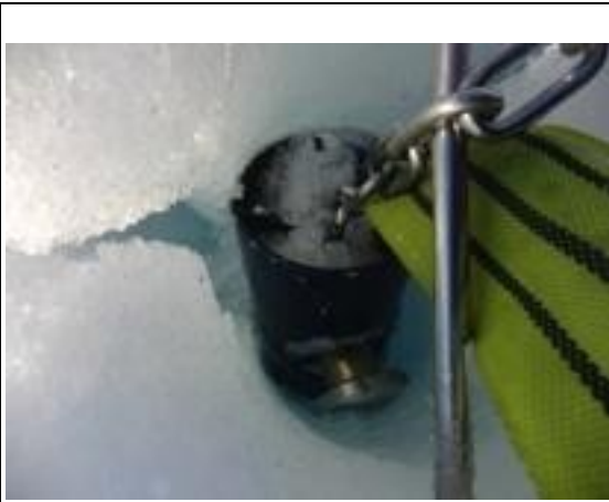
Figure 4.12: The boreholejack head. Here it can be seen that the piston is extended and the ice has cracked.
