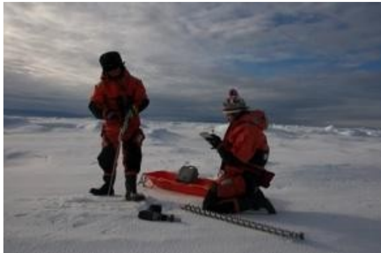
Fig. 4.3: Liqiong and Ella measuring snow and ice thickness at a calibration drilling.
