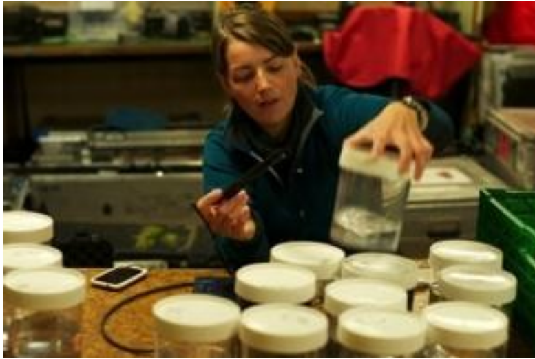
Fig. 4.4: Salinity measurements of melted ice core samples onboard Lance.
