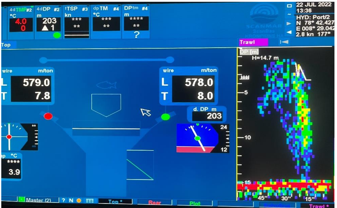
Figure 16. Screen of Scanmar Scanbas monitor with school of capelin entering the opening of the Vito pelagic trawl at TR-1 west of Svalbard on 22 July 2022.
