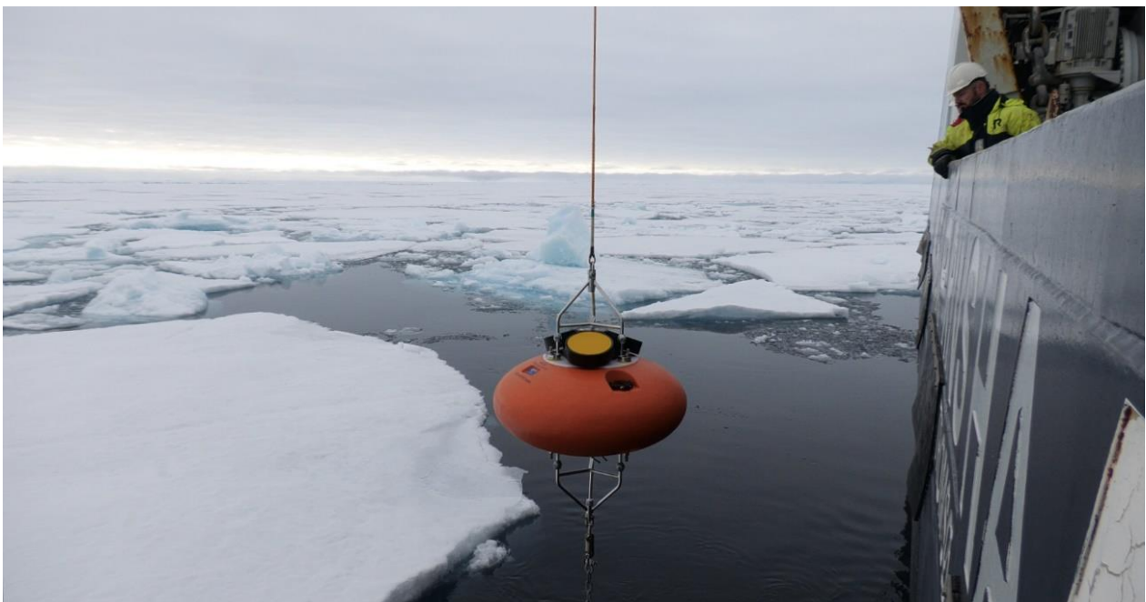
Figure 26. The Signature55 ADCP going in the water by the Amundsen-1 site (Photo: Trine Lise Sviggum Helgerud/NPI).
