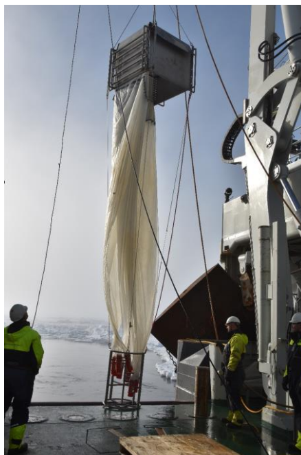
Figure 22. Mammoth net used for sampling of mesozooplankton.
