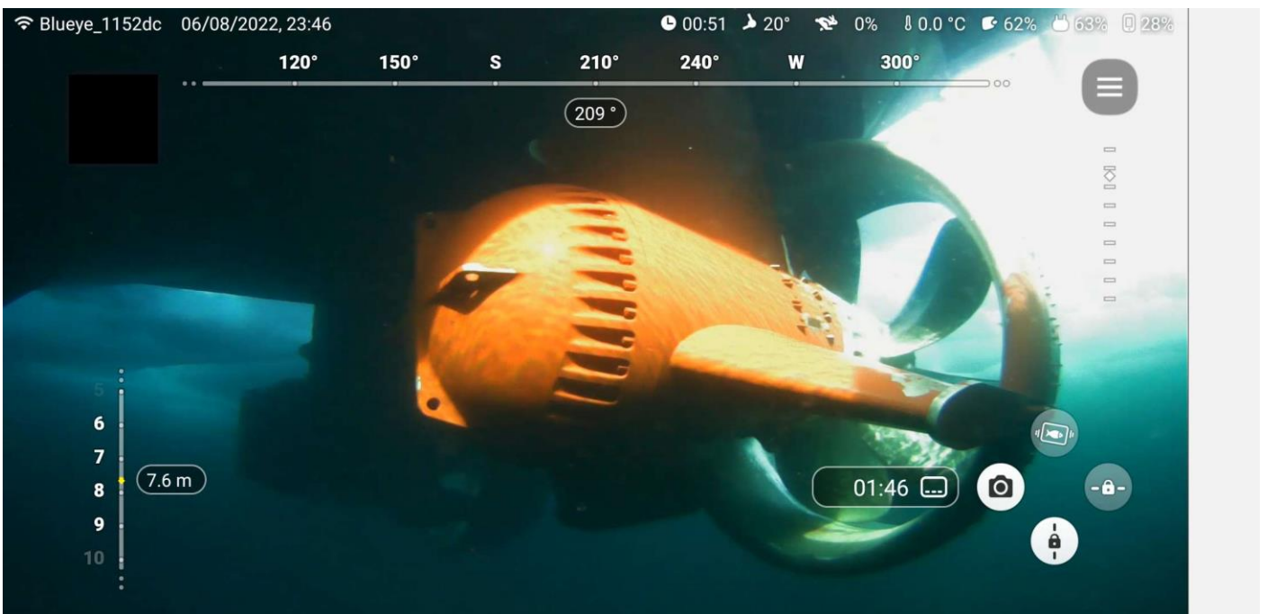
Figure 56. Before retrieving the vehicle, and because navigation with the Hipap system was reliable, the was used to inspect the propellers at the aft of the vessel.
