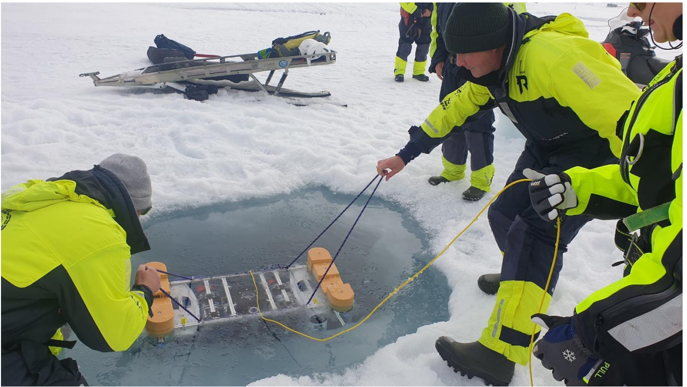
Figure 55. The DBE was the largest device on the cruise that needed to be deployed through the ice. Building a hole for ice was time consuming and required several people.
