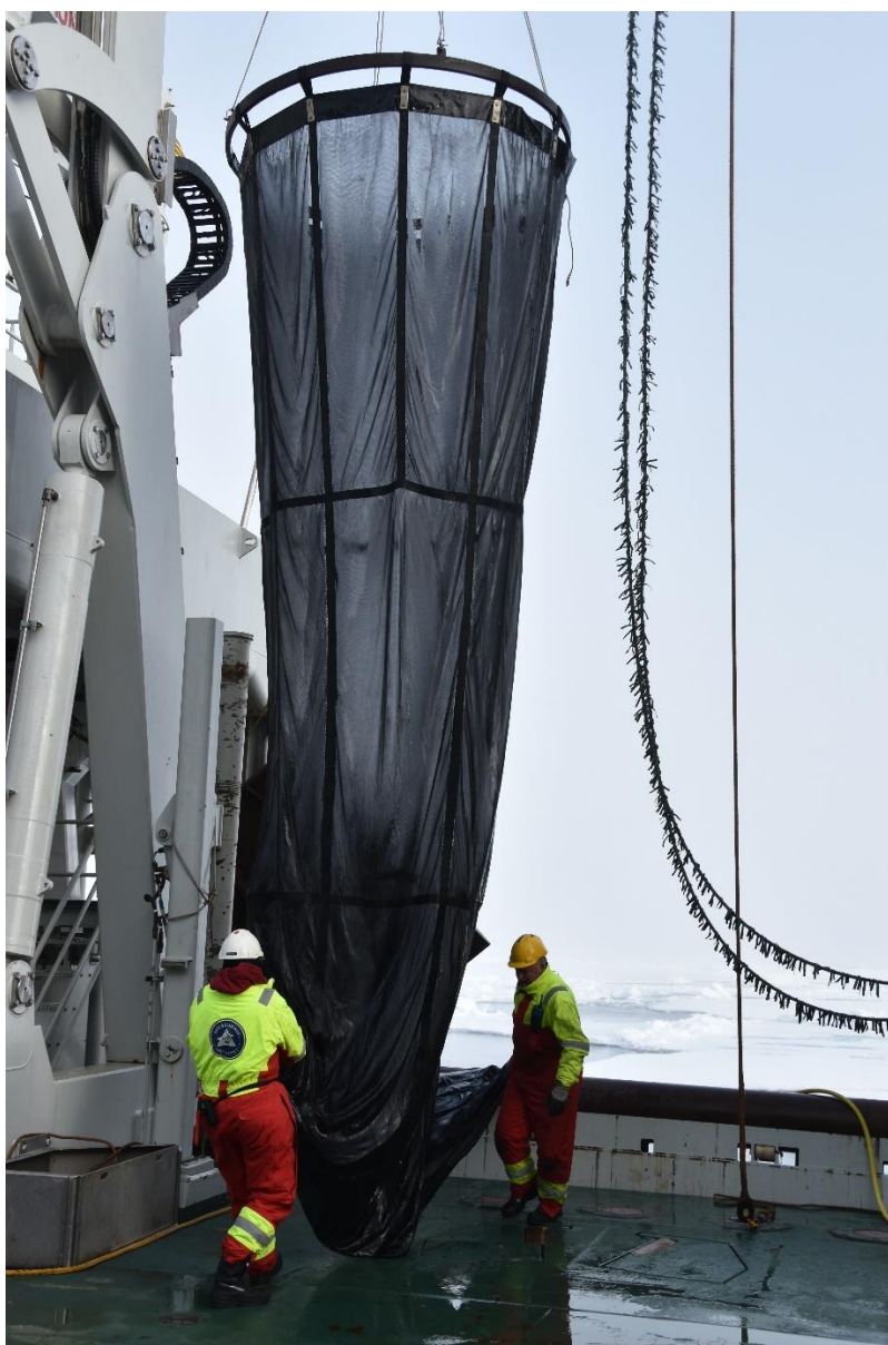
Figure 23. MIK net used for sampling of macrozooplankton.
