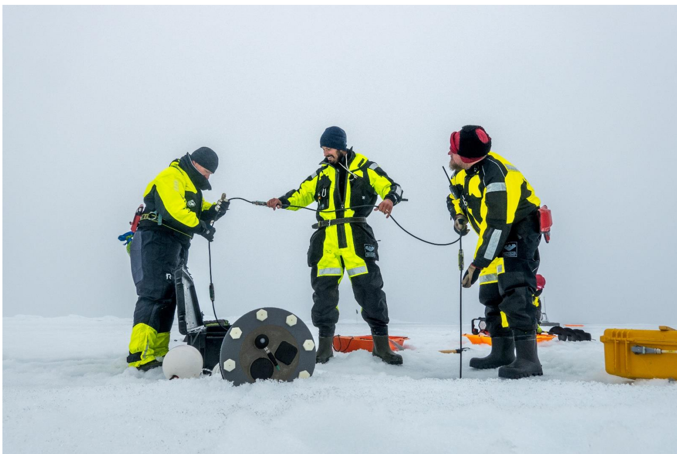
Figure 53. Marius Bratrein, Pedro De La Torre and Mats Granskog place carefully the long sensor chain through 1.6m thick ice. The PAR sensor, GPS and Iridium antennas on the top of the floating buoy are shown. A SIMBA is placed next to the instrument and left to drift together. (Photo: Trine Lise Sviggum Helgerud/Norwegian Polar Institute)
