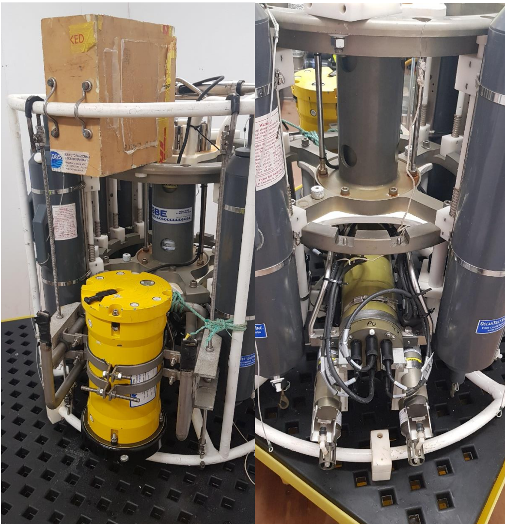
Figure 7.1: Pictures of the LADCP and buoyancy mounted correctly on the “labelled” side of the rosette and the two-lined sensor package sticking far out on the “unlabelled” side to maximize space.
