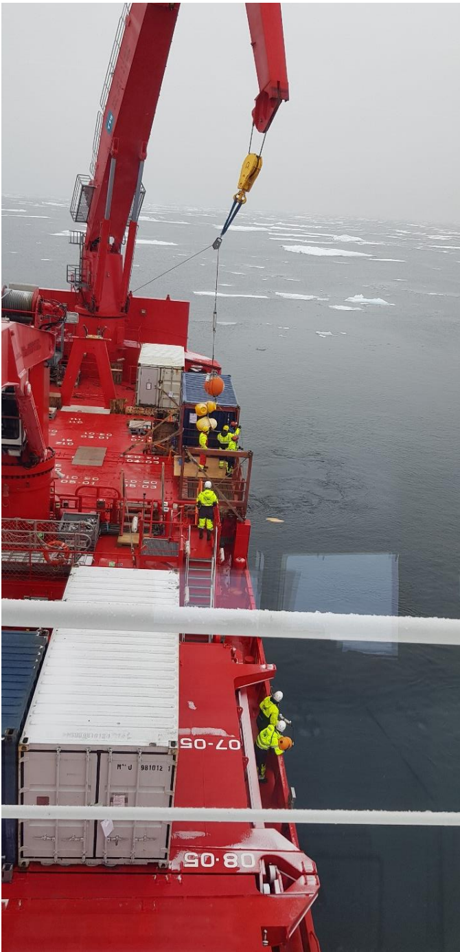
Left: Lifting of the top float group of F10 with the main crane over the side of the ship from the flat-rack platform. The seal wire of the weak-link is laid out along the side of the ship with people manually managing the instrument and float atop during the deployment.
