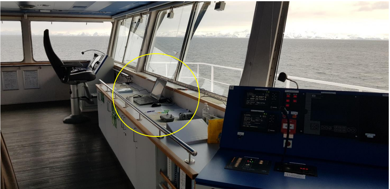
The NPI navigation computer conveniently located on the bridge for displaying sea ice maps in QGIS together with the ship's real time position. Position data were obtained and logged as cruise track via an RS232 NMEA feed from the ship's GPS that was installed for that purpose before the departure.
