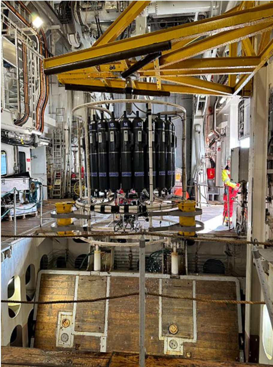
Figure 7. The main 24-Niskin bottle rosette coming up through the moonpool after a completed cast. The CTD sensor package is visible in the center of the rosette, and the two yellow ADCPs on the sides. Photo by Ann Kristin Balto.
