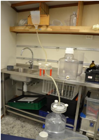
Figure 16: Filtration setup for filtered seawater used in the dilution experiments.
