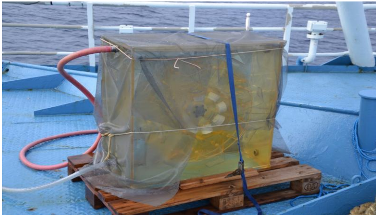
Figure 17. Plankton wheel covered with screens to mimic ambient light levels in the surface layer.
