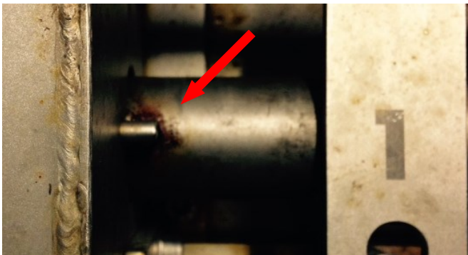
Figure 12: There is a small pin on the rotating cylinder which should point straight at the pin seen here.
