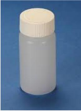
Figure 6: Acid washed 20 ml plastic scintillation vials used for nutrient samples.
