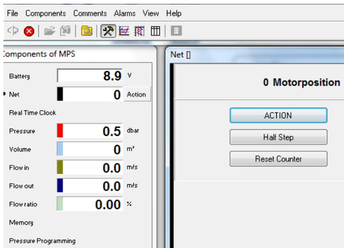
Figure 15: Mark *Net* in the right menu and use *Half step* to reset rotating cylinder
