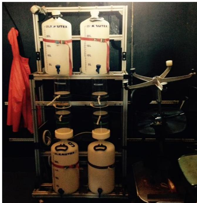
Figure 8: Filtration tower to concentrate microplankton samples
