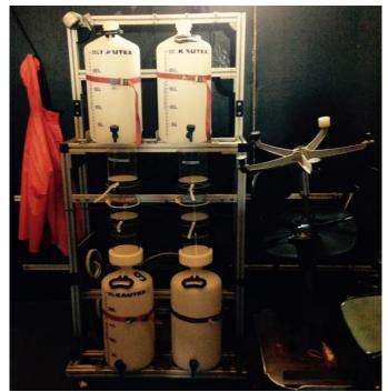
Figure 8: Filtration tower to concentrate microplankton samples
