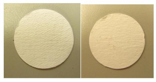
Mesh side – PARTICLES ON THIS SIDE. Soft "wave" side – back side.
